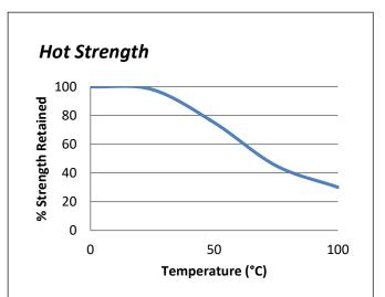
Fully cured lap shear specimens conditioned to pull temperature for 30 minutes before testing at temperature.
