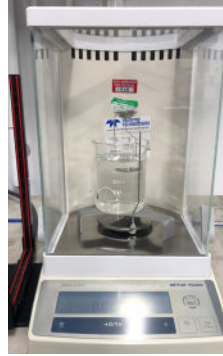
Figure 2. Balance fitted with a density determination kit
