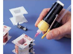
Wetted parts of the 752V hand-lever valve are made from UHMW polyethylene, making this an ideal choice for dispensing CAs in low-volume production processes.
