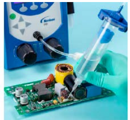
The Ultimix II provides the most control when dispensing watery CAs.
