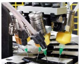
Install dispense valves in-line for high volume production.
