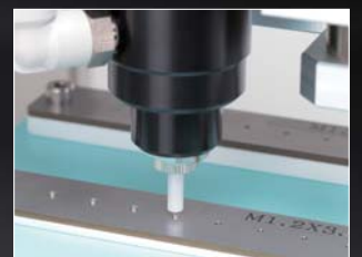
Tightens screws as small as M1.0.
